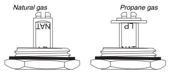
To convert the regulator snap the device out of the top and refit the other way up. The snap in converter device is marked to show which gas it is set for. Make sure the device is secure in the top cap and refit the cap to the regulator.
